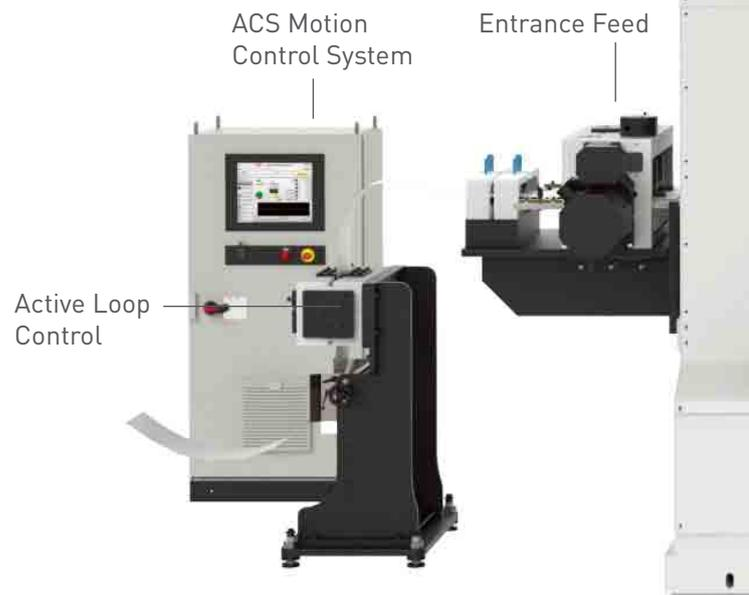
**1 Quantum Active Loop Control** delivers reduced material acceleration in coordination with feed roll motion to reduce loop whip while increasing production speeds and accuracy.
